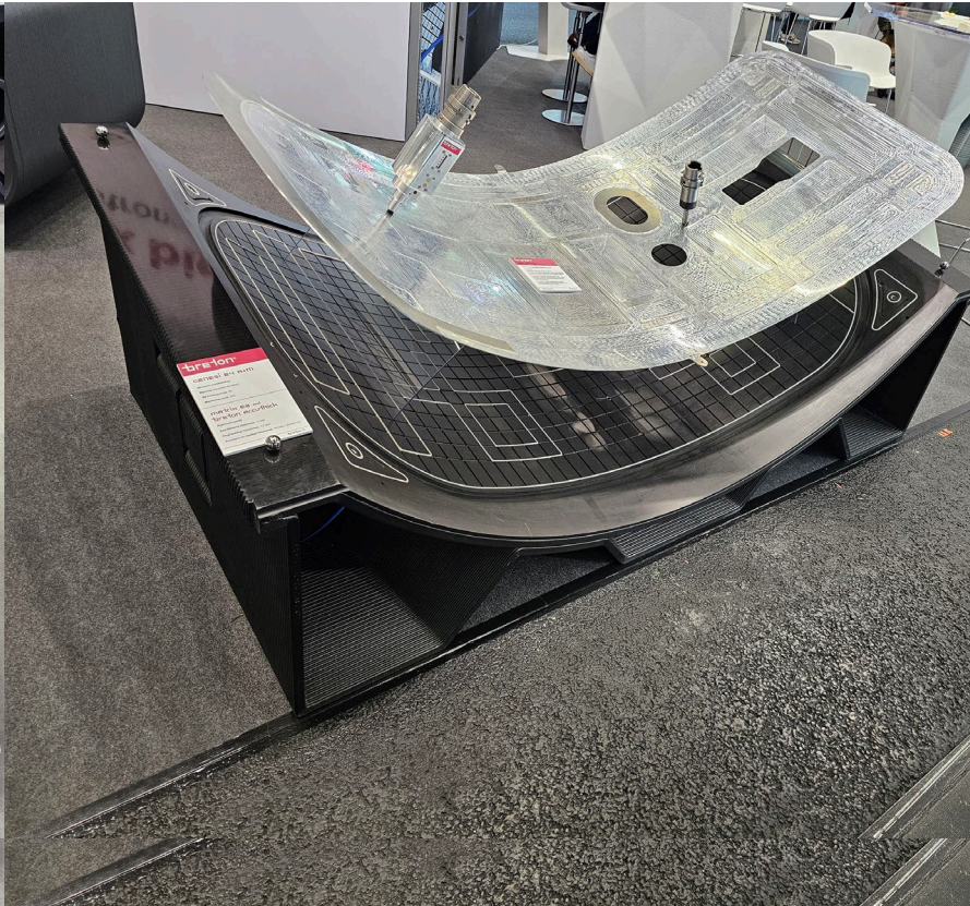
Breton: Vacuum workholding Material: Recycled PC+25CF, Print time: 9 + 20 h
